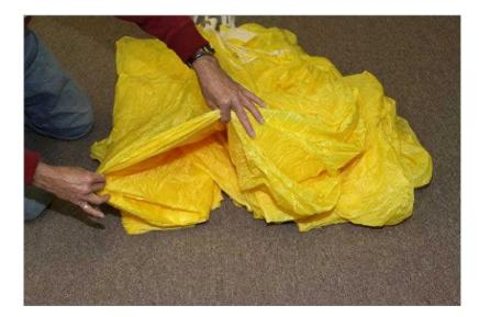
Flake the material between the C and D lines away from the line channel in the center of the pack job. Make sure the D lines are grouped together and stacked neatly on top of the A, B and C lines. It is important to keep even tension on all the line groups throughout the remainder of the pack job. Pulling on the "T" seams directly above the line attachment point will keep the lines straight and maintain the folds in the material.
