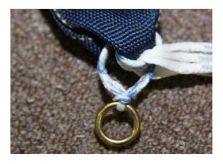
9. Rotate the whole Wrap-It Link so that the ring is located in the riser end.
