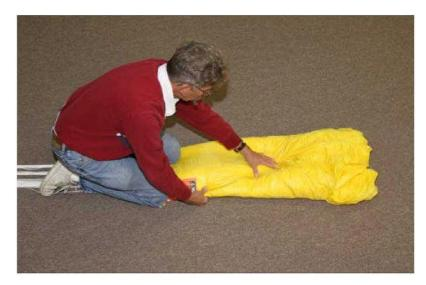
Kneeling on the lower tail, pull the top of the folded reserve up onto your lap. make sure the seven leading edge openings are exposed and the tail is not wrapped in front of the openings.
