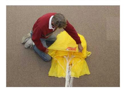
Pull up the slider by grabbing the tapes around its center and walking from the connector links to the base of the folded canopy.
