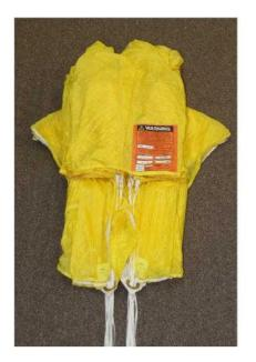
Carefully "S" - fold the nose under the canopy, making sure the leading edge remains exposed, but does not extend past the edges of the folded canopy.
