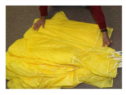
Repeat the previous step to flake the material between the B and C lines.
