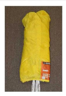
Fold the bottom of the folded reserve back and on top of itself making approximately a six inch "S"- fold
