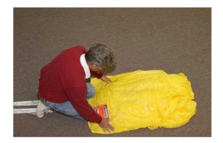
Tuck the center tail panel around the canopy, working from bottom to top and making sure not to cover the leading edge.
