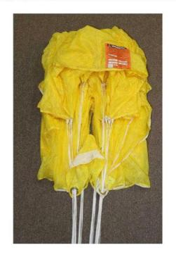
Quarter the slider, dividing the material evenly between the slider grommets. Make sure the slider grommets are seated against the slider stops sewn into the stabilizers.
