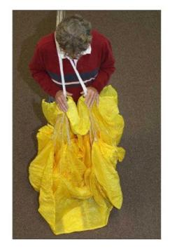
Flake the nose of the canopy. Pull each cell completely out. Pick up the next cell taking care not to miss any of the seven cells.
