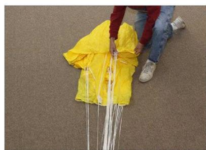
Lay the center cell of tail on top. It should be spread out to the same width as the rest of the folded canopy.
