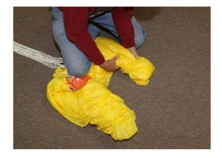
Lay the canopy in its side until all seven "T" seams are straight from leading edge to trailing edge as shown.
