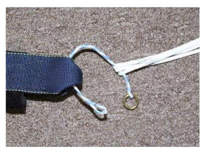
2. Feed the loop end of the Wrap-It Link through the lines again, second time.
