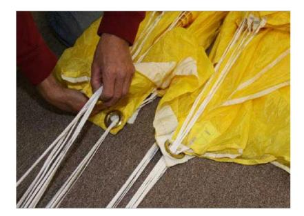
Fold in half the fold between the A and the B lines and the folds between B and C lines to narrow the pack job.
