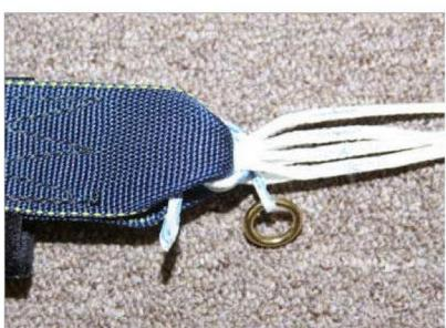
6. Feed the loop end of the link through the other end of the link (through the same loop with the ring).
